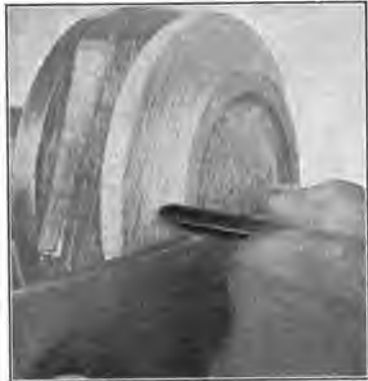
Fig. 128. Scraping with Round Nosed Tool.
